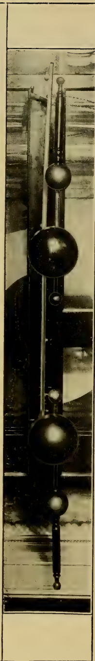
PLATE 22.—Author's Short-Circuit Stick. In the lower figure the stick is laid on the poles and shunts the current from the tube. In the upper figure the operator is seen lifting it from the poles to let the current excite the tube for the required exposure-time. See text for full description.
